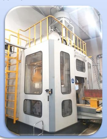
production of different cores for easy and complex inner structure in castings
