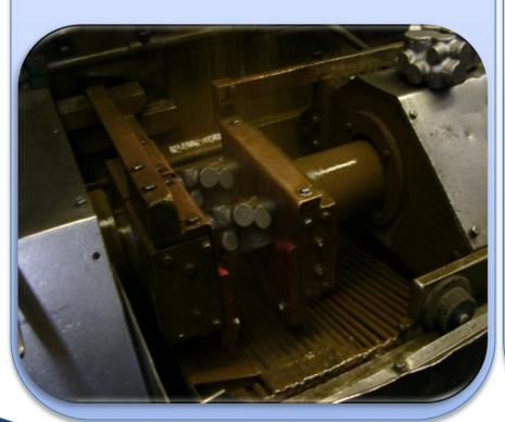
Showering the components with test liquid while magnetizing them, followed by a visual inspection under UV light
